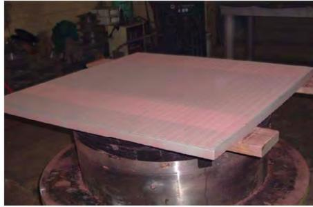
Cook Legacy applied Jacquelyn™ Coating to vertical traveling screens constructed by Banker Wire. The screens, now biofouling-resistant, are strong and environmentally sound. The use of Jacquelyn™ allowed for the durability of stainless steel with protection similar to that of 90-10 CuNi.
