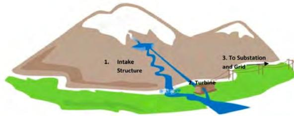
Coanda Power systems are modular and consist of proven technologies. They use Coanda intake screens that catch only the bottom layer of water — allowing clean water to pass through and fish and debris to pass over. The systems can be built in remote areas with limited civil structure and little or no existing power supply. Coanda Power is an achievable, sustainable, and simple solution to meeting energy needs.
